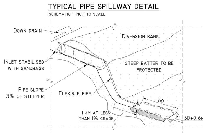
TYPICAL PIPE SPILLWAY DETAIL SCHEMATIC - NOT TO SCALE
